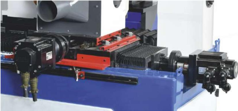
Dual Servo driven grinding operation
