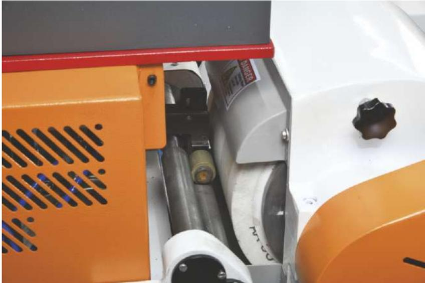
Fully automatic grinding of ring frame cots
