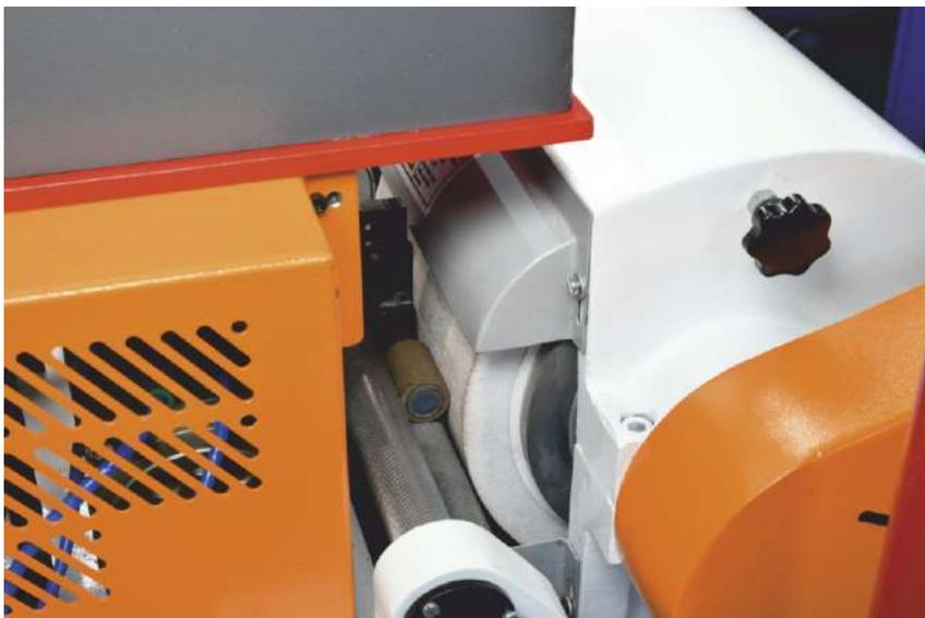
Fully automatic grinding of speed frame cots
